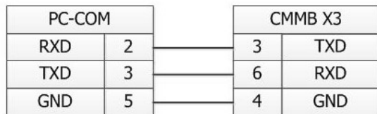
Figure 10-1: Communication wiring between PC (DSub 9-pin) and CH-23 controller
