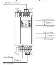
Figure 4-4 Cable routing distance
