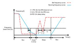
When the set frequency is lower than the frequency lower limit, and the ones place of P01.19 is set to sleep, the VFD stops according to the tens place of P01.19 and sleeps once running at the lower limit for the time specified by P01.34. If the set frequency exceeds the lower limit again and it lasts for the time specified by P01.20, the VFD restores to the running state automatically and increases to the set frequency.
