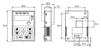
Figure D-3 Keypad openings without a bracket
