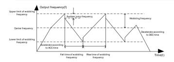
Wobbling frequency = Central frequency (Set frequency) x P08.15 (Amplitude of wobbling frequency)
