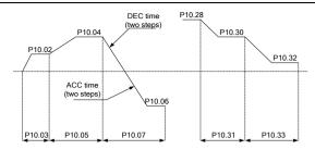
Note: The sign of multi-step speed determines the running direction of simple PLC, and a negative value means reverse running. ACC time means the time needed if the VFD speeds up from OHz to the max. output frequency (P00.03). DEC time means the time needed if the VFD speeds down from the max. output frequency (P00.03) to OHz. Select corresponding ACC/DEC time, and then convert 16-bit binary number into hexadecimal number, finally, and then set corresponding function codes.
